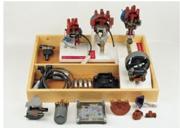
Order No. 1215 Ignition model case
